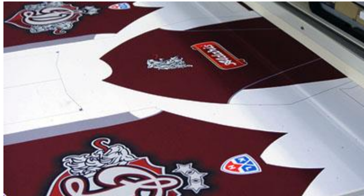
Figure 34 Laser contour cutting sportswear on a conveyer flatbed.
