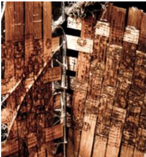
Figure 101 left image of a woven laser etched veneer trapped in resin (Own work)
