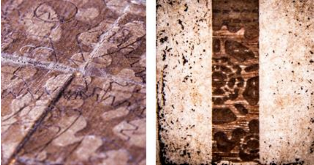
Figure 92 on left woven recycled grey card with vector and raster engraving.
