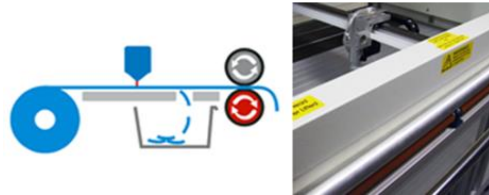
Figure 35 Conveyor system feeding rolls of fabric to and from the laser bed.
