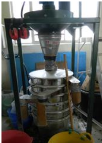
Figure 56 Machine used for crushing the glass. Picture taken at interview.
