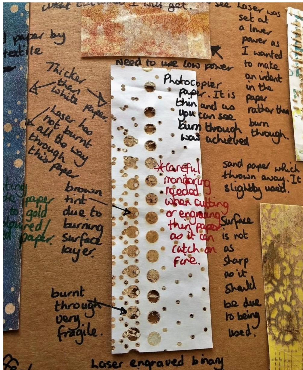
Figure 79 Initial experimentation onto different surfaces documented in a scrapbook as evidence of practice. To be utilised as a visual reference to how materials react to the impact of laser engraving and cutting (Own work 2015)
