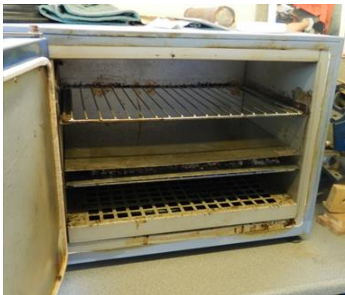
Figure 76 Industrial oven used in schools to soften and remould plastics. (Own image, 2014).
