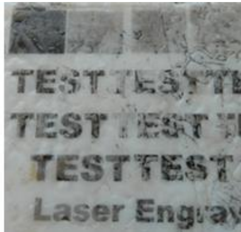
Figure 106 Fused crisp packets with plastic compound. Chemical black marked.
