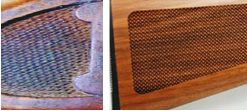
Figure 30 Hand Engraved checkering and Figure 31 Laser machine engraving on gun stock using gravel chisels and vice. ( www.epiloglaser.com )
