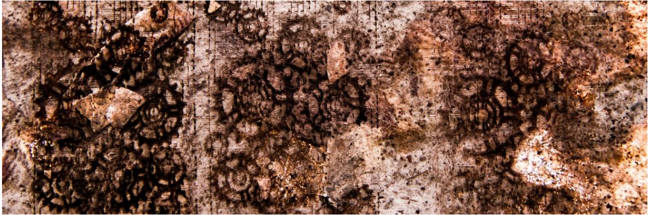
(Figure 96) Organic materials and recycled pulp made from mixed paper such as newspaper and old reading books. Laser engraved at different speeds and power with various laser focus heights. Own work
