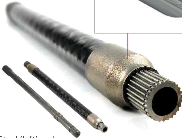
Steel (left) and carbon-titan shift (right)
