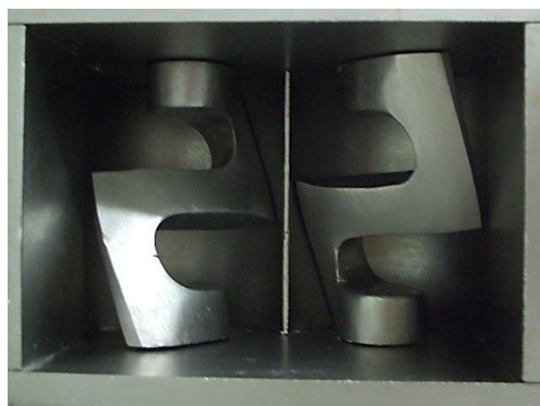
Figure 1.2 The Z blade mixer
