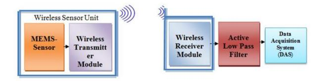
Figure 3.2 Wireless sensing system block diagram.
