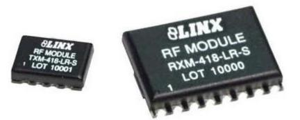
Figure 3.1 RF transmitter and receiver modules(Linx, 2009 R, 2009 T).
