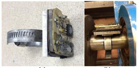
(a) (b)  $U_{58g} = 58 \times 10^{-3} kg \times 15 \times 10^{-3} m = 870 \times 10^{-6} kg.m$   $U_{58g} = 870 \times 10^{-6} kg.m \times (148.7)^2 = 19.24 N$ Where: (148.7 rad/s) is the maximum rotor speed
