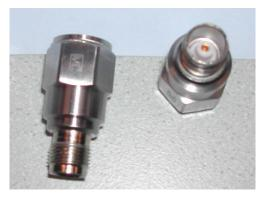
Figure 5.9 SINOCERA accelerometers
