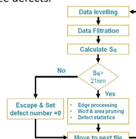
Figure 4. Computing model of data handling method
