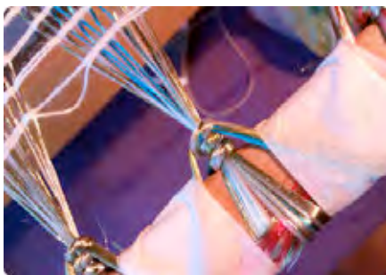
3. Fixing monofilament onto cloth roller
