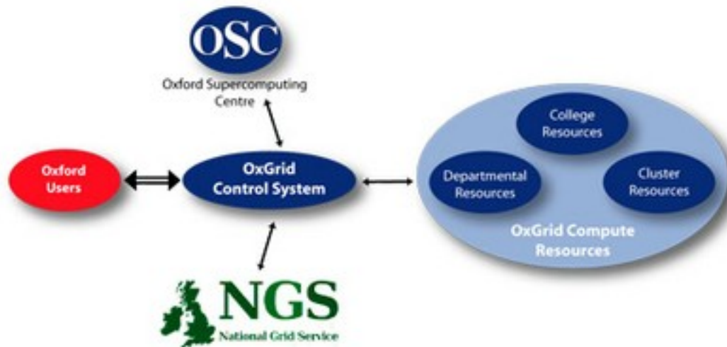
Figure 2.4: OxGrid Diagram (Wallom & Trefethen, 2006)
