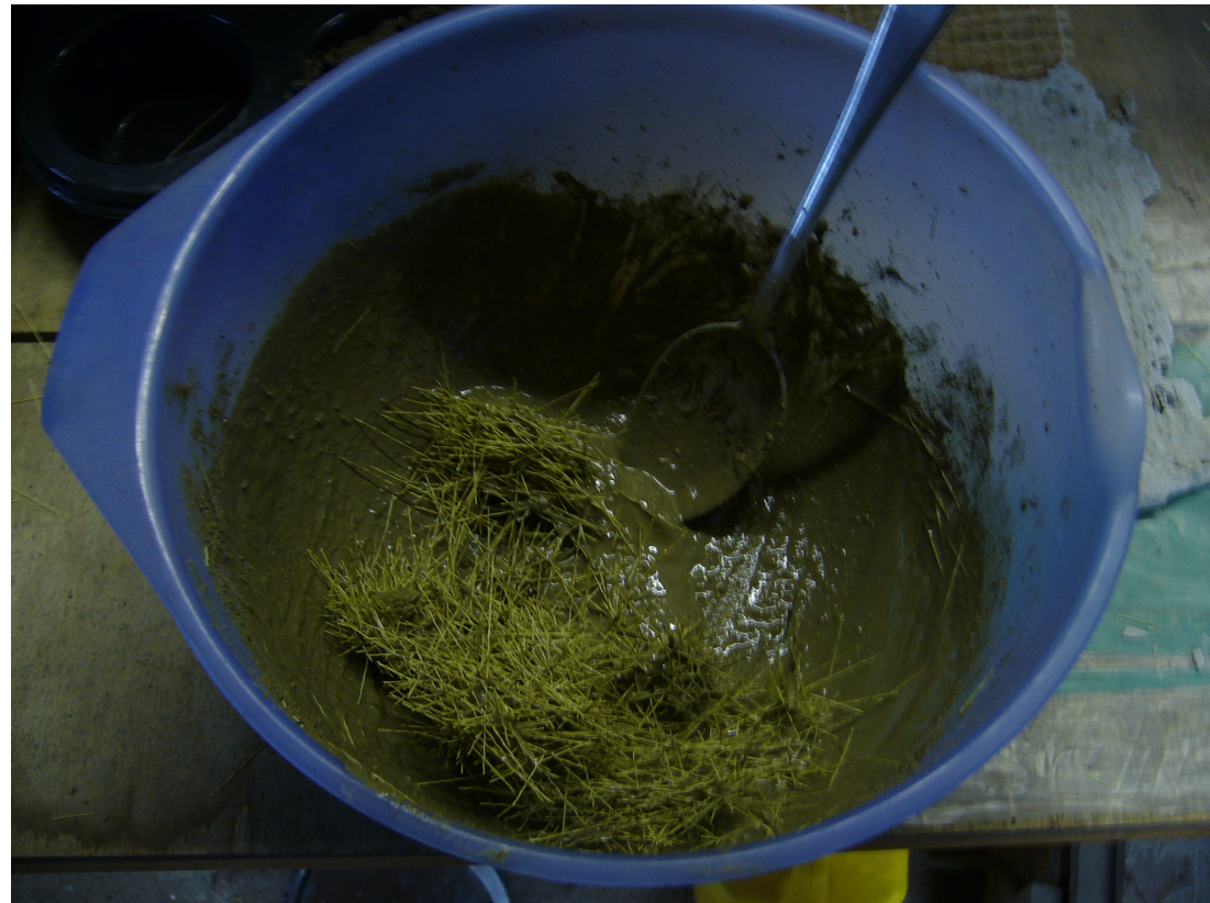
Image 75. Method 3. Mixing of concrete and nylon fibres
