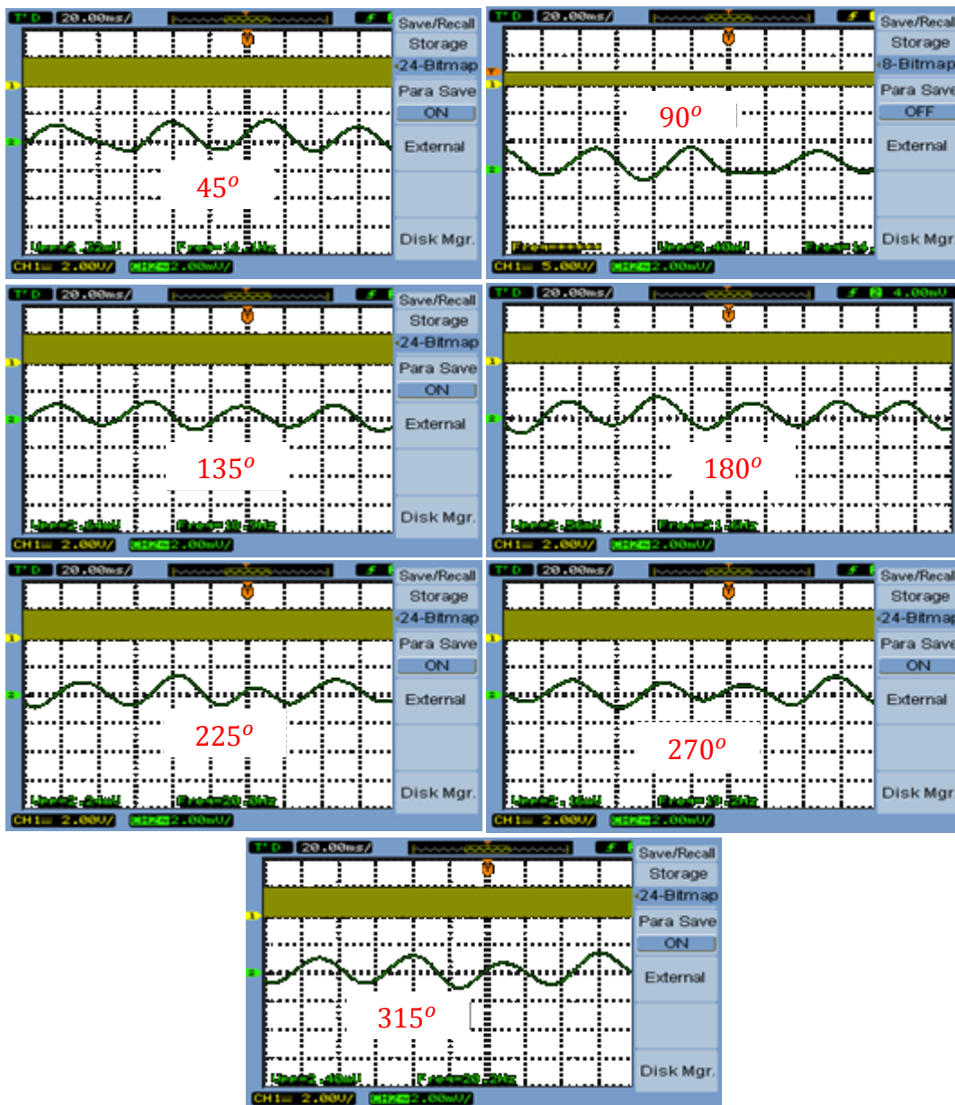
Figure 4.23: Practical results of 8-PSK and the attenuation of the DAC at 20 Hz
