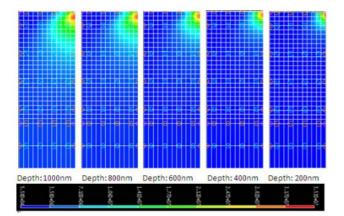
Figure 10b Effective Stress Distribution for Coating with  $4\mu m$  Thickness and 5GPa Modulus of Elasticity
