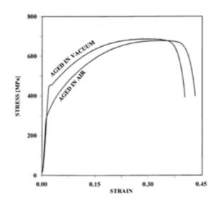
Figure 1: Relationship between stress and strain [5]
