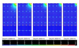
Figure 11a Effective Strain Distribution for Coating with  $5\mu m$  Thickness and 5GPa Modulus of Elasticity
