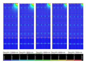
Figure 13a Effective Strain Distribution for Coating with  $6\mu m$  Thickness and 5GPa Modulus of Elasticity
