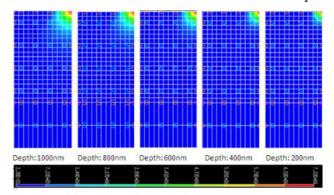
Figure 10a Effective Strain Distribution for Coating with 4µm Thickness and 5GPa Modulus of Elasticity
