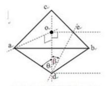
3-side pyramidal indenter tip-  $\Delta$ abc is an equilateral base -  $\beta = 53.4^{\circ} \pm 0.5^{\circ}$  -  $\theta = 69.6^{\circ} \pm 0.5^{\circ \circ}$ ~0.1-1 µm tip radius-
