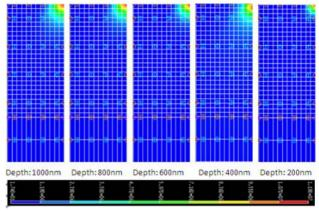
Figure 12a Effective Strain Distribution for Coating with  $6\mu m$  Thickness and 5GPa Modulus of Elasticity
