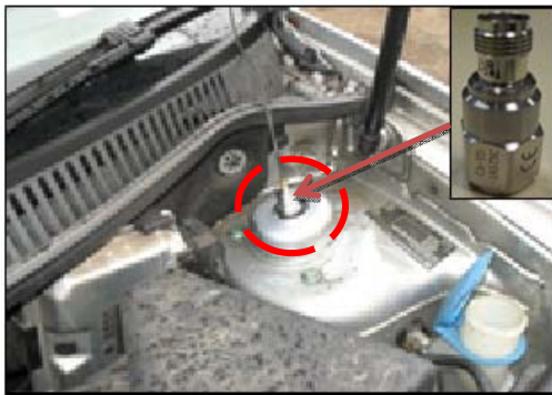
Figure 3. IEPE Accelerometer fixed on the top of front left suspension
