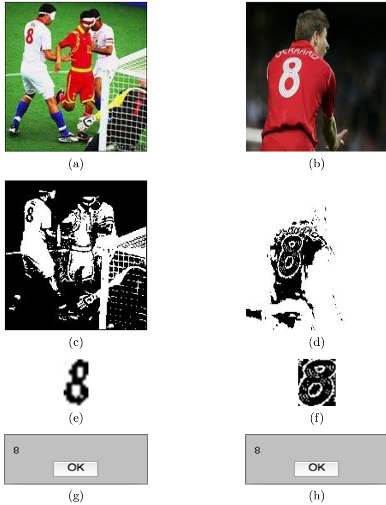
Fig. 2. Examples of results obtained with our OCR system. First row: input image. Second row: segmented image. Third row: extracted character. Fourth row: recognized character.
