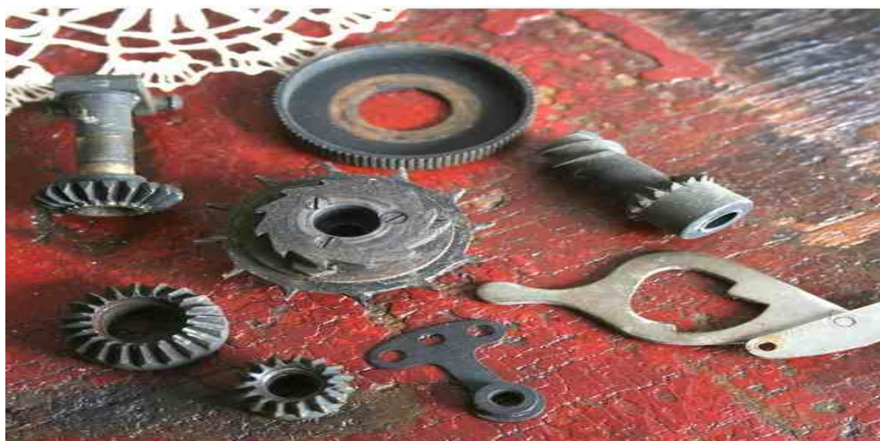
Figure 20: Parts of a vintage typewriter, the angle-threaded bolt is what this author believes to be an example of a typewriter bolt
