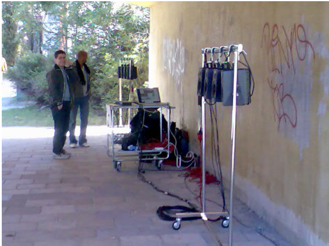
Figure 2.3 - In the foreground 4 of the 8 speakers hanging from a mobile coat rack. In the background the other 4 speakers and in between the two sets of speakers a computer running the installation software and a pressure zone microphone used for our motion detection software.
