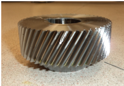
a) 30% tooth breakage
