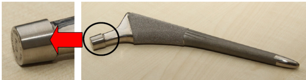
Figure 12. Total hip replacement femoral stem with highlighted micro-threaded taper surface.
