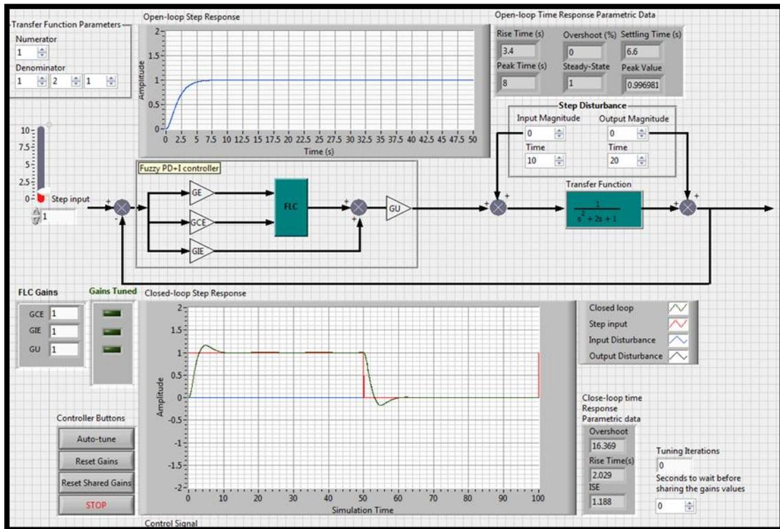
Figure 2. Front Panel View of the FLC.
