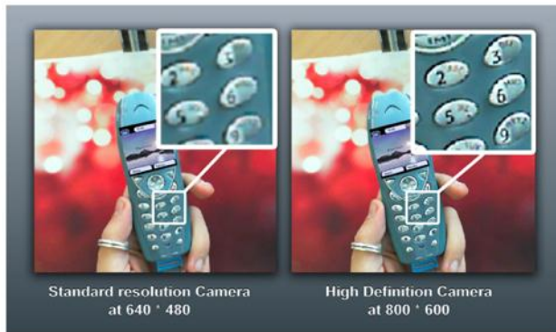
Figure 4: Detail of the prototype keyboard as displayed on the screen using a regular and HD camera.
