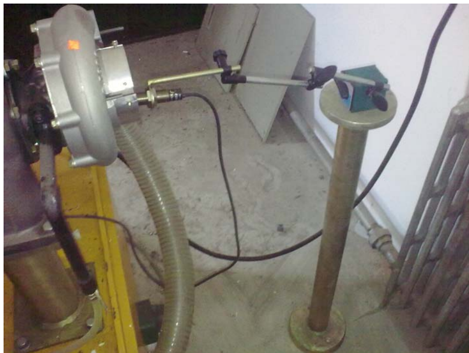
Figure 7. 11. The rotational speed sensor fixed on a universal bracket
