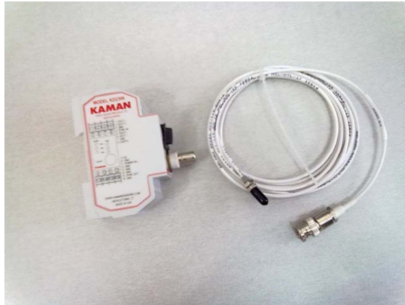
Figure 7. 7. KAMAN KD2306 1U1 eddy current displacement transducer
