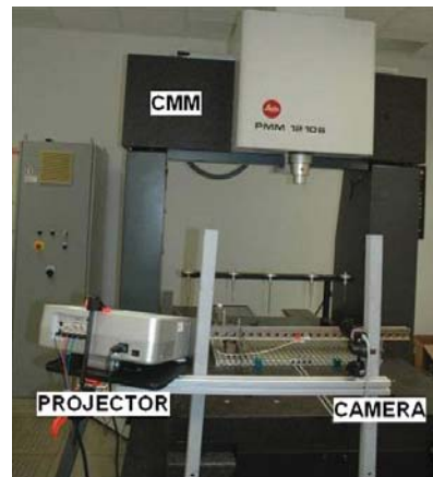
Figure 3: Hybrid fringe projection and CMM system
