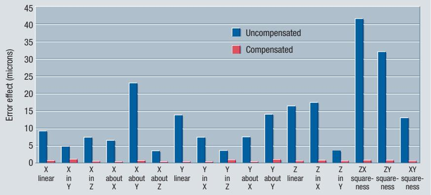
The historic measure of the accuracy of a machine, namely axis accuracy, is being replaced by volumetric accuracy as the understanding of machining errors increases. This understanding is driven mainly by manufacturers – particularly the aerospace industry – undertaking 5-axis work on large machines.
