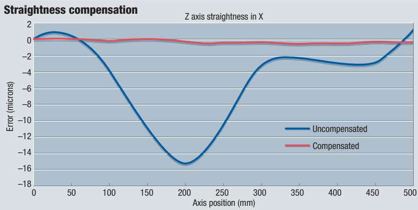
any 3-axis machine based upon calibration data. The software not only outputs a single-value figure for the volumetric accuracy, but also indicates the most significant error sources.
