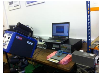
Figure 14. The photo of PEC thermography set-up
