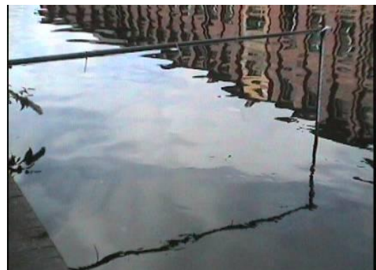
Figure 7: Pole holds thermocouples probe and flow meter
