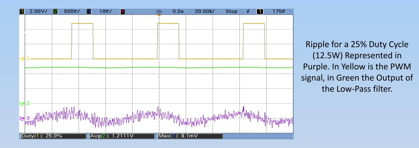
The power ripple of the load is represented in the figure above. Displayed in Purple is the dissipated power with AC coupling to allow an easy display of the ripple. The main ripple frequency is approximately 15.5 kHz which is the frequency of the PWM signal. The maximum measured ripple for a 25% duty cycle is 80mW which is ±6% error. This value is acceptable for RES testing.
