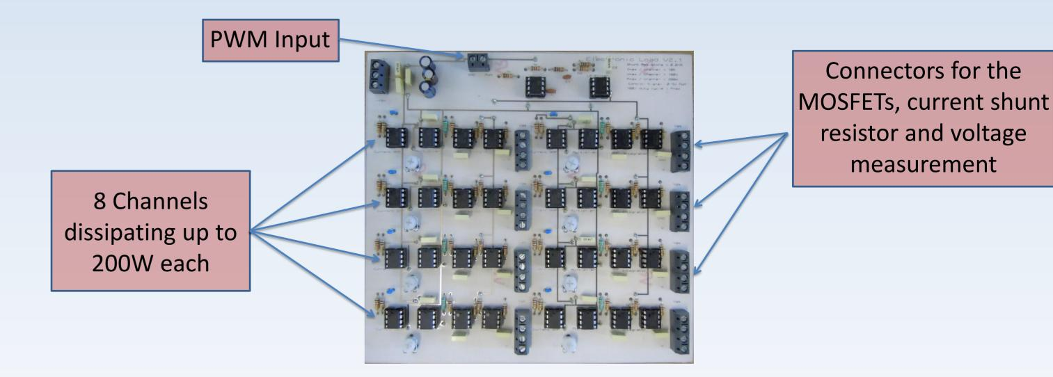
Picture of the improved electronic load control circuitry capable of dissipating 1.6kW
