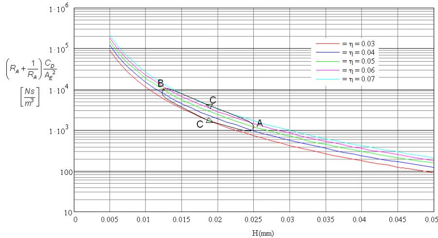
Figure 3.2 Graph showing bearing damping against bearing gap
