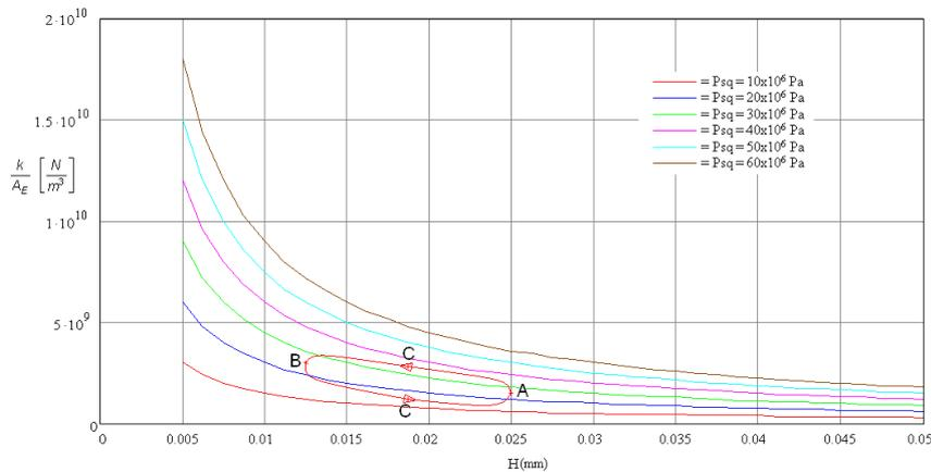
Figure 3.1 Graph showing bearing stiffness against bearing gap
