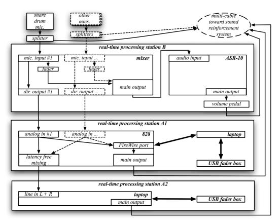
Figure 2: The *abstr/cncr* tour setup signal flow
