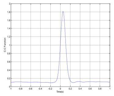
Figure 4: velocity result of a bell moving inside ICC flow meter time daily = 0.9s and Vb=0.055 m/s
