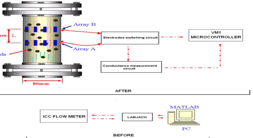
Figure2 : VM1 control the electrode circuit.
