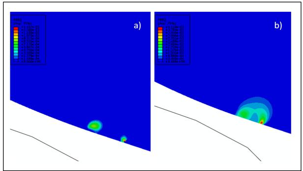
Figure 4: Plastic strains (PEEQ) when V-band clamp is taken off flanges after axial clamping load of 60kN has been applied, a)  $\mu$ =0, b)  $\mu$ =0,2
