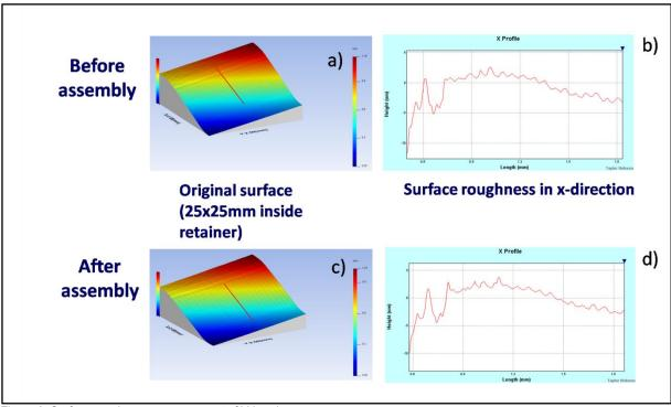
Figure 6: Surface roughness measurement of V-band
