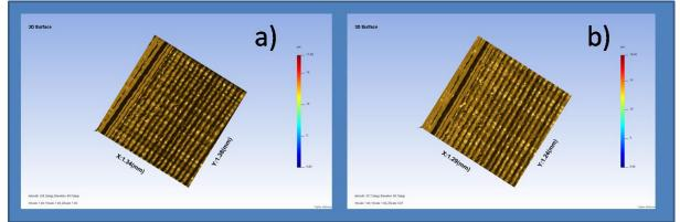
Figure 7: Surface measurements after levelling, a) before and b) after assembling
