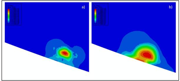
Figure 2: Residual stresses when V-band clamp is taken off flanges after axial clamping load of 60kN has been applied, a)  $\mu$ =0, b)  $\mu$ =0,2
