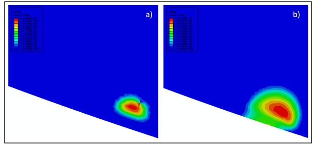
Figure 3: Plastic strains (PEEQ) when V-band clamp is taken off flanges after axial clamping load of 30kN has been applied, a)  $\mu$ =0, b)  $\mu$ =0,2
