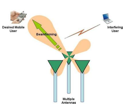
Figure 1: Diagram of the beam-forming technique
