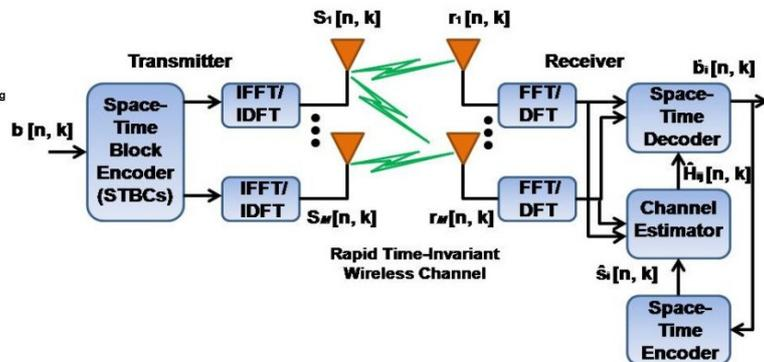
Figure 2: Schematic diagram of the MIMO-OFDM system
