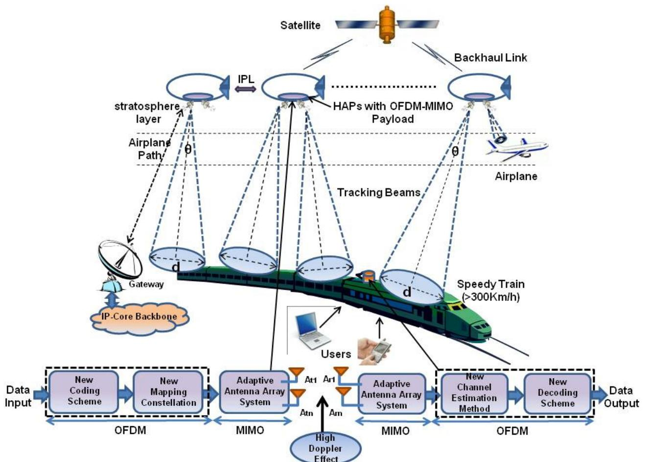
Figure 3: Hybrid OFDM-MIMO-HAPs-Satellite System
