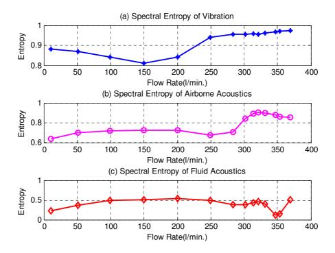
Figure 6 Spectral entropy of vibration, airborne acoustic and fluid acoustic spectra
