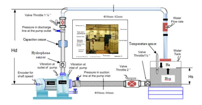
Figure 1 Schematic of pump test system
