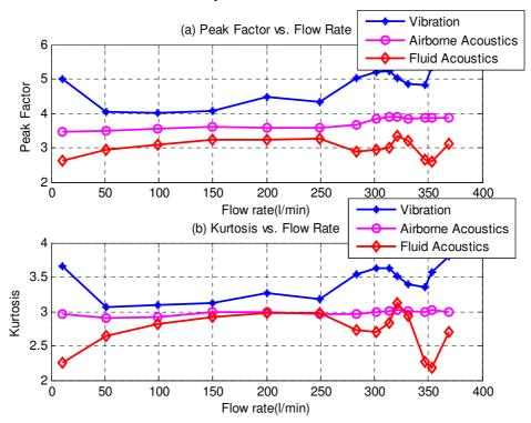
Figure 3 Conventional dimensional parameters vs. flow rate
