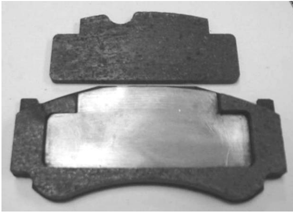
Figure 7 – View of pad and insert before pressure film is fitted. Note smooth metallic face for film bed.
