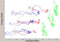
**Right:** To quantify the mass flow fluctuation a ratio of  $m_{max}/m_{min}$  was used. This ratio was then plotted on the graph against both average pressure ratio and average corrected mass flow.
