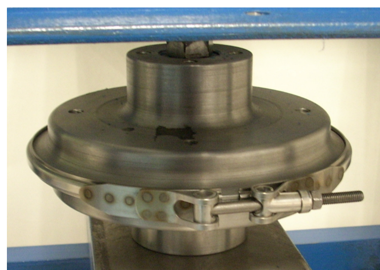
V-band retainer assembled to circular pair of flanges
