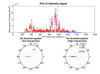
Peak detection of the mean value of the intensity and split of signal in low and high frequencies
