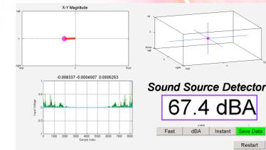
Real time display of the Acoustic Intensity
