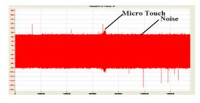
Figure 2: Raw signal showing micro-touch detected by AE sensor
