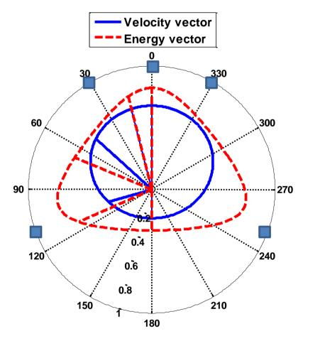
This above gain response **is not** suited to an irregular 5-speaker layout. It results in a poor \* velocity vector and energy vector response (see right).
