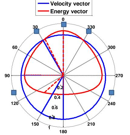
This change results in velocity vector and energy vector magnitudes which 90 are closer to an ideal value of 1 and vector angles which match more closely the intended directions (see angles at 0, 30, 90, 150 and 180 degrees).
