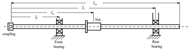
Figure 2: Ball screw arrangement
