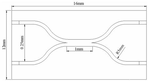
Figure 6: The dimension of the IO coupler
