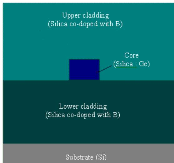
Figure 7: The structure of the coupler waveguide
