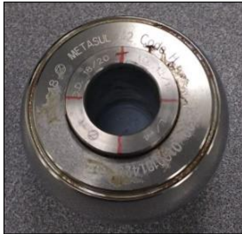
Figure 119: Retrieved femoral head with a visual reference mark on the underside of the component. Cross mark indicates the 'front' azimuth position of the femoral head.
