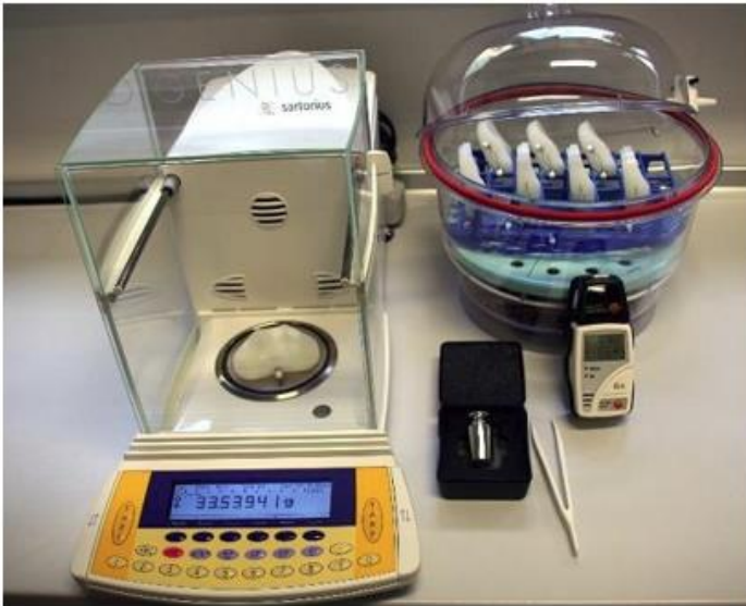
Figure 43: Gravimetric measurement method. Weighing of a polymer knee component [133].
