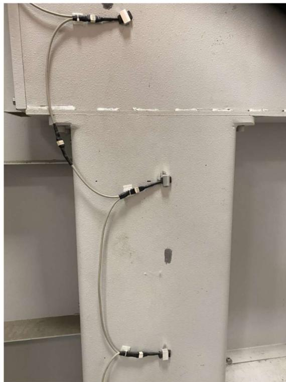
*Figure 5.8 Three DS18B20 temperature sensors mounted on the CNC machine frame.*
