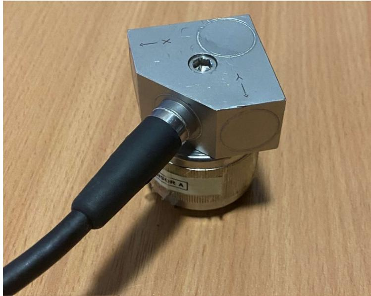
*Figure 5.3 Tri-axial accelerometer used for model calibration and testing*
