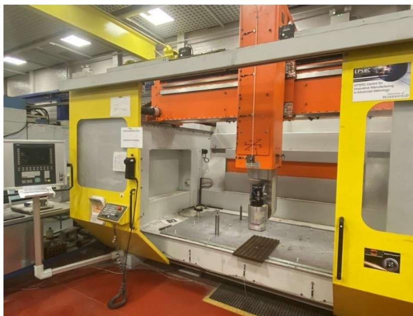
*Figure 5.1 The 5-axis gantry-type CNC machine used in this study*
