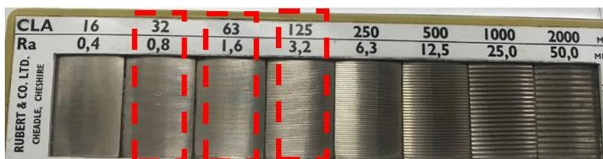
Figure 4. 8 Standard part manufacturing by turning for dichotomous classification
