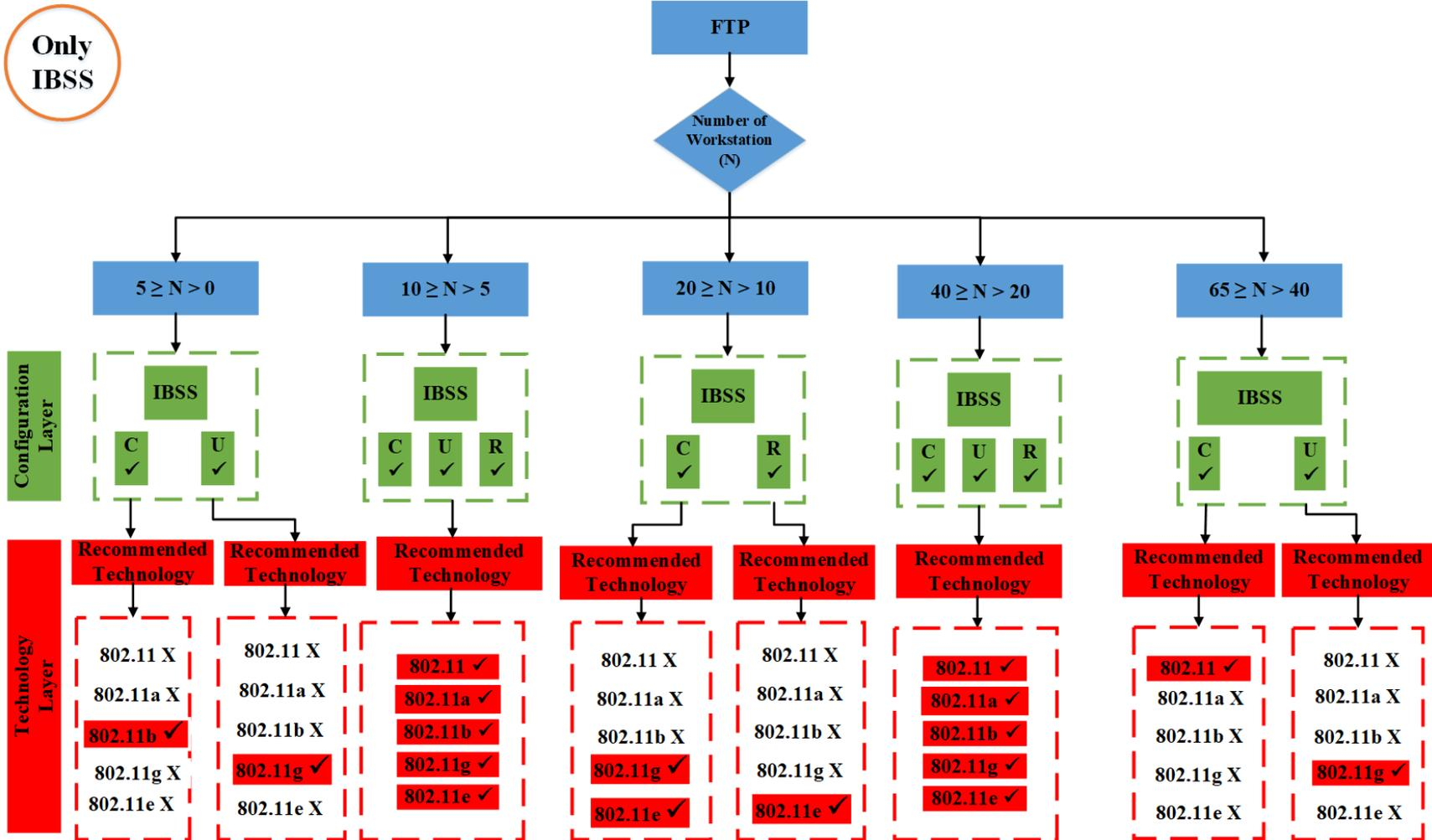
Figure 5. 8 Flowchart of only IBSS's results for FTP
