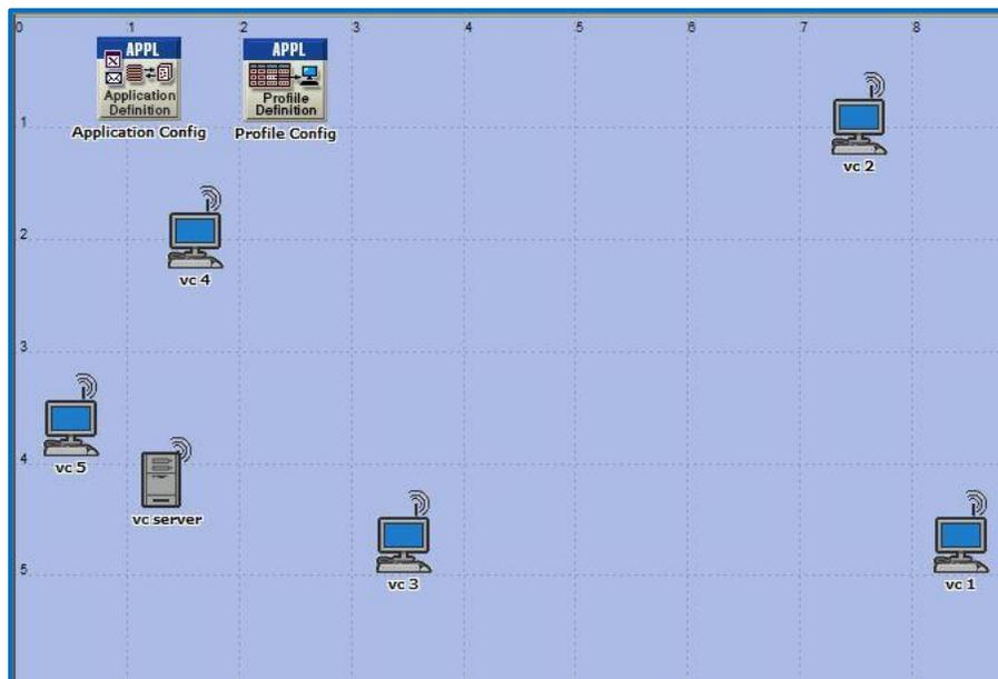
Figure 4. 9 Five Workstations Randomly distributed in IBSS Configuration
