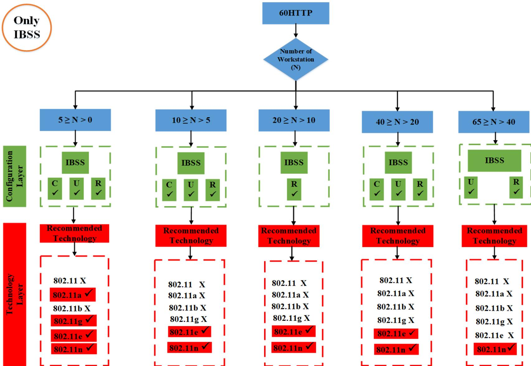
Figure 6. 22 Flowchart of only IBSS's results for 60HTTP
