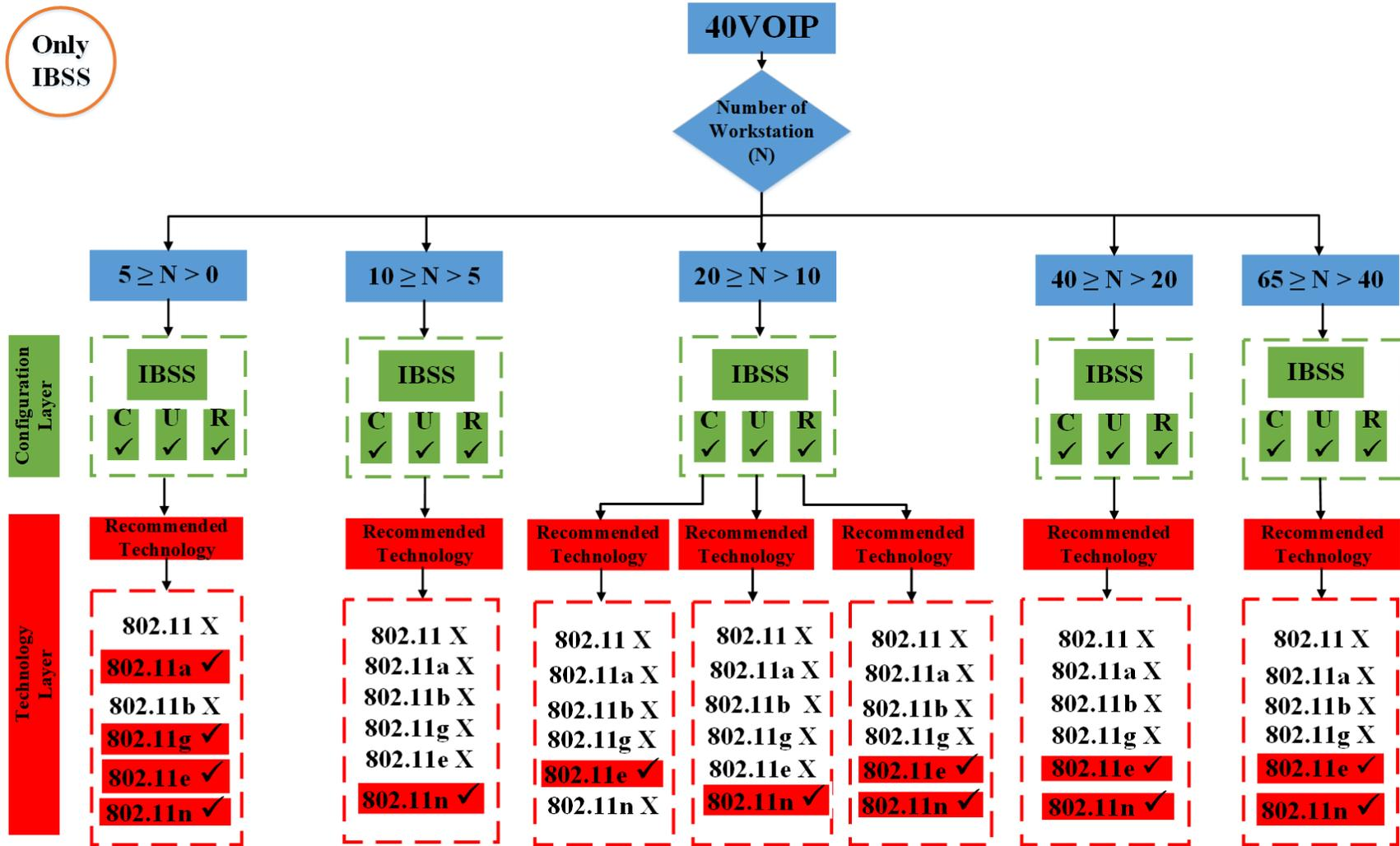
Figure 6. 28 Flowchart of only IBSS's results for 40VOIP
