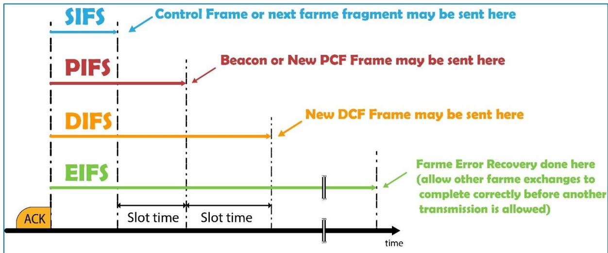
Figure 2. 8 Inter frame Spacing (Refaet, Amed, Abed, & Aish, 2020)
