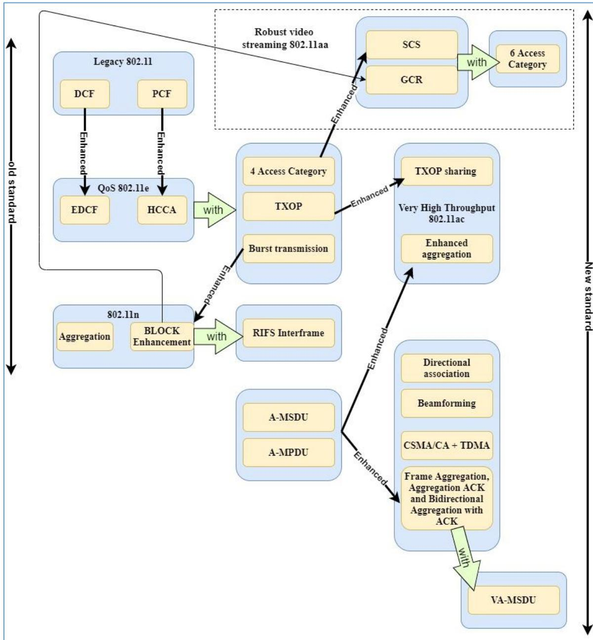
Figure 3. 3 IEEE 802.11 enhancement mechanisms (Zawia, Hassan, & Dahnil, 2018)
