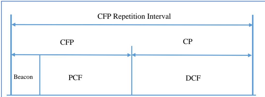
Figure 2. 9 CFP repetition interval (Refaet, Amed, Abed, & Aish, 2020)
