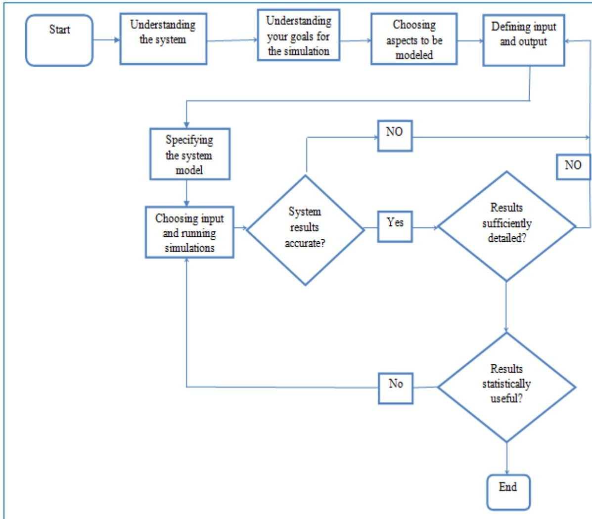
Figure 3. 5 Proposed Technique Simulation Flow Chart
