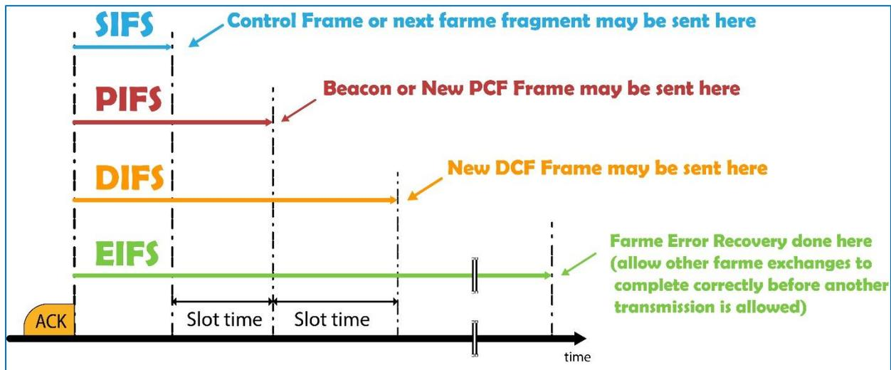
Figure 2. 8 Inter frame Spacing (Refaet, Amed, Abed, & Aish, 2020)
