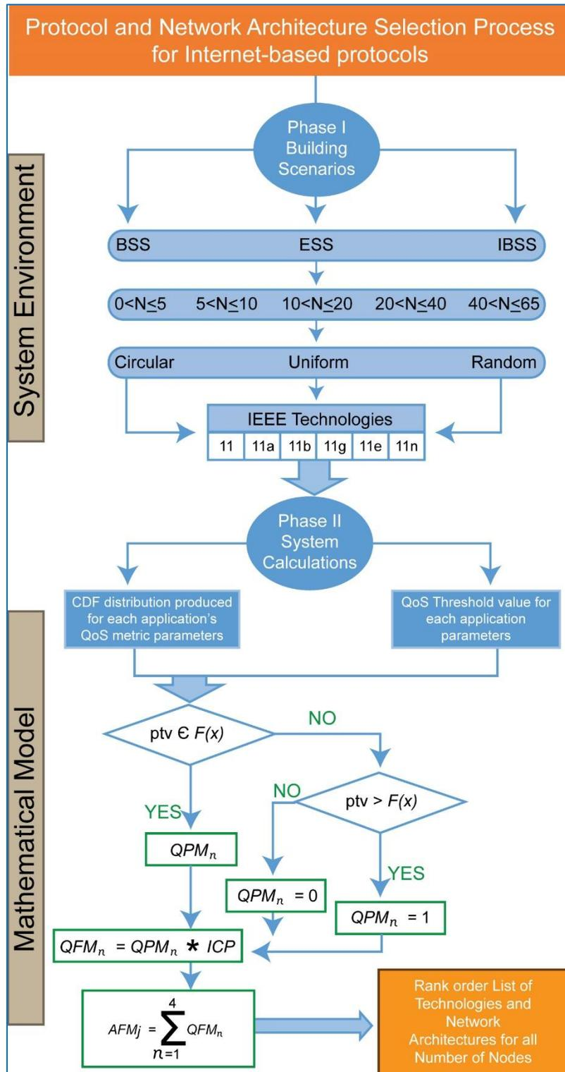
Figure 3. 34 Flow chart of Research Algorithm Process
