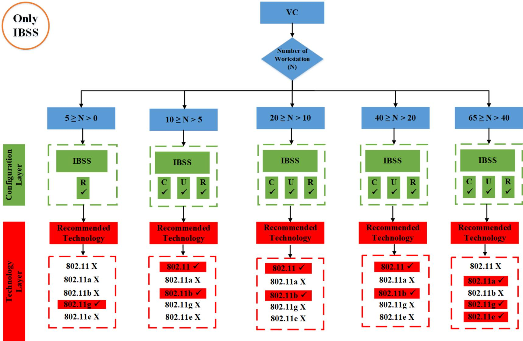
Figure 5. 4 Flowchart of only IBSS's results for VC
