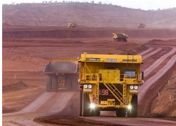
Figure 20: A fleet of driverless trucks operating on a mining site in Western Australia (Dodgson, 2016)
