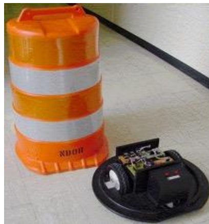
Figure 15: A robotic safety marker unit (Farritor and Rentschler, 2002:1)
