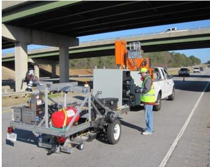
Figure 16: An automatic crack identification and repairing system (Georgia Tech, 2012)
