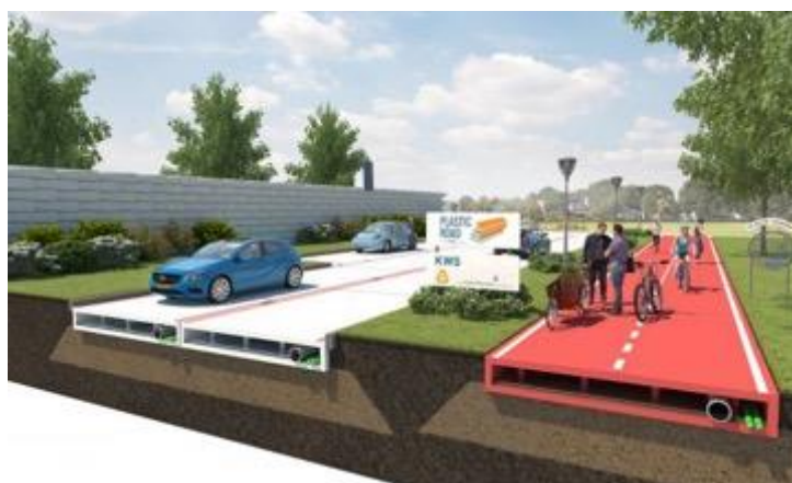
Figure 21: Concept of prefabricated plastic slabs (VolkerWessels, 2015)
