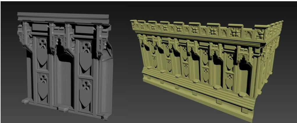
Figure 7. Completed sections with symmetry and with corner elements added.
