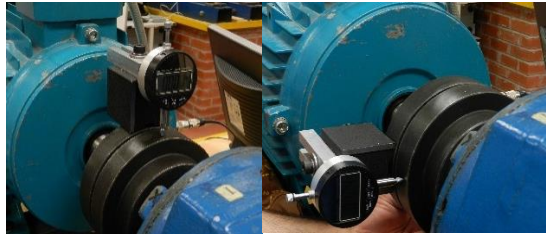
Figure 4.5 Digital dial indicator for shaft alignment (author)
