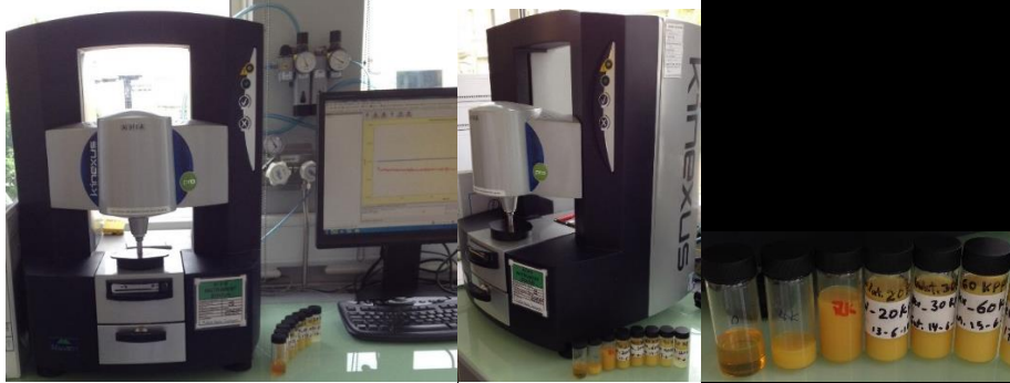
Figure B.1 the viscosity rotary meter
