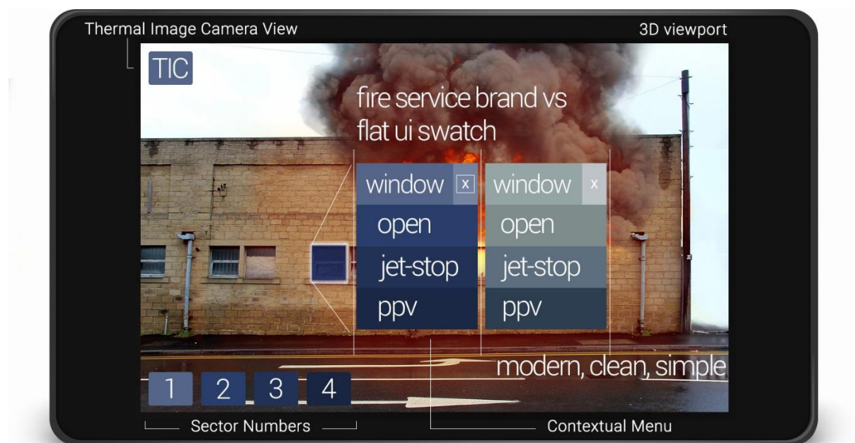
Figure 21: A design idea trialling colours, adding the TIC (Thermal Imaging Camera) button and replacing the action bar with a contextual menu.
