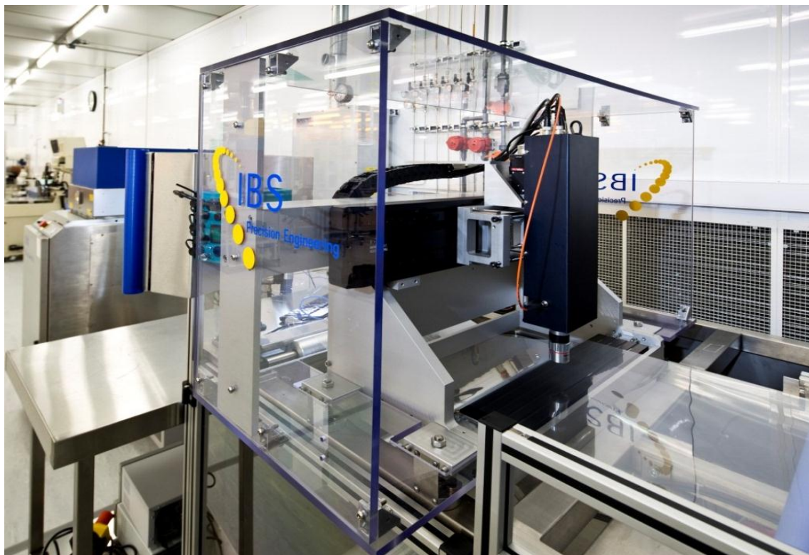
Figure 8-8: WSI system implemented as a demonstrator for R2R barrier films inspection
