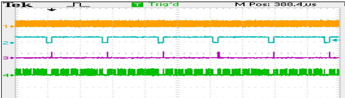
Figure 8.23 The DiPPM Coder Waveform Multi Codewords Output
