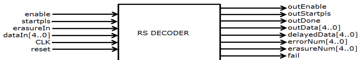
Figure 6.25 RS(31,23) decoder top block view
