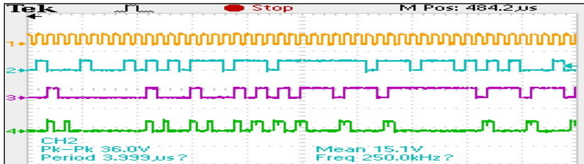
Figure 8.26 The System Transmitter Waveform Single Codeword Output
