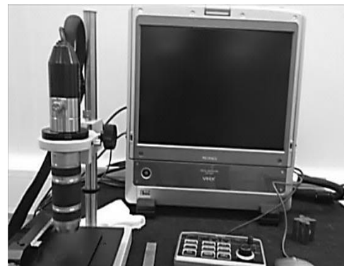
Fig. 6 Pin/disc wear scar measurements by using digital microscope (VHX)
